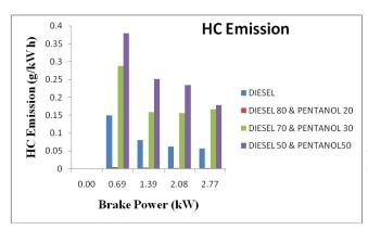
By this observation the HC emission for diesel fuel is constant but the diesel and pentanol blended fuel is varies corresponding to the ratio of blend the HC emission is keep on decreasing when the brake power increased.
