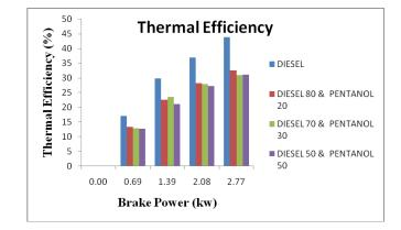
In the observation the blended diesel and pentanol fuel the thermal efficiency is decreasing.
