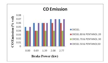
By this observation the Co emission for diesel fuel is constant but the diesel and pentanol blended fuel is varies corresponding to the ratio of blend the 2:1 ratio blended fuel emits more Co emission.
