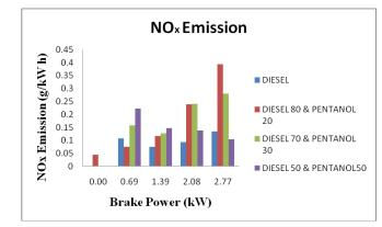
By this observation the NO<sub>x</sub> emission for diesel fuel is increasing at full load but the diesel and pentanol blended fuel is varies corresponding to the ratios; the blended ratio of 10:3fuels emits moreNO<sub>x</sub> emission than the diesel, at the full load condition of diesel and pentanol blends the NO<sub>x</sub> emission decreased.
